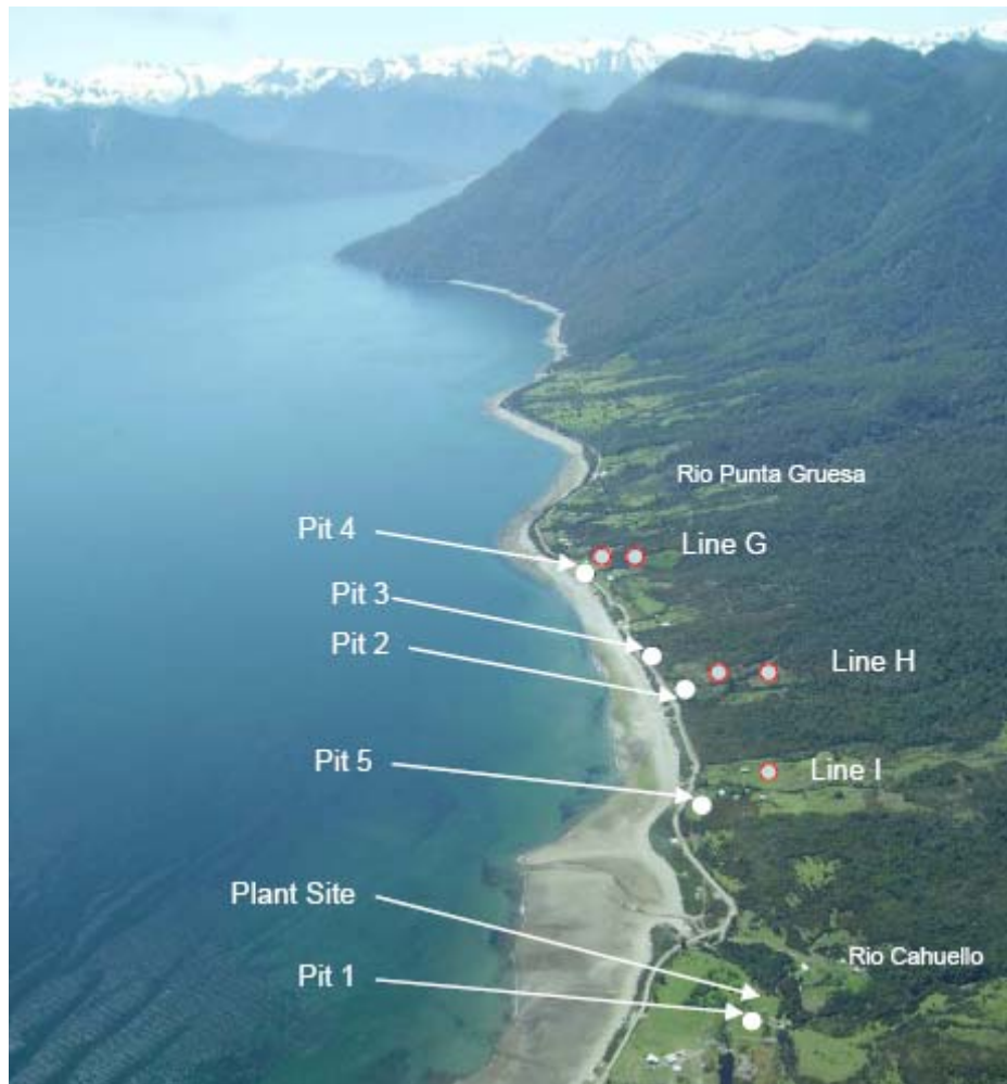
Figure 1. The white circles represent the sites of the pits dug in May 2007. The red circles are the sites of the 1931 pits. The new pitting programme will concentrate on Lines H and I.
