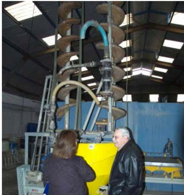
Figure 1: The spirals and shaking table being used to recover the heavy mineral concentrate in the sample treatment laboratory in Santiago.
