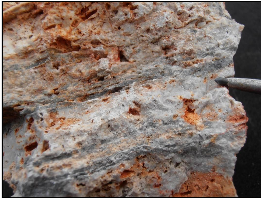
Figure 2: Close up of advanced-argillic (alunitic) and acid-leached overprint on earlier porphyry-style banded veins. Note corroded texture parallel to vein banding. (Photo: N. Callan)
