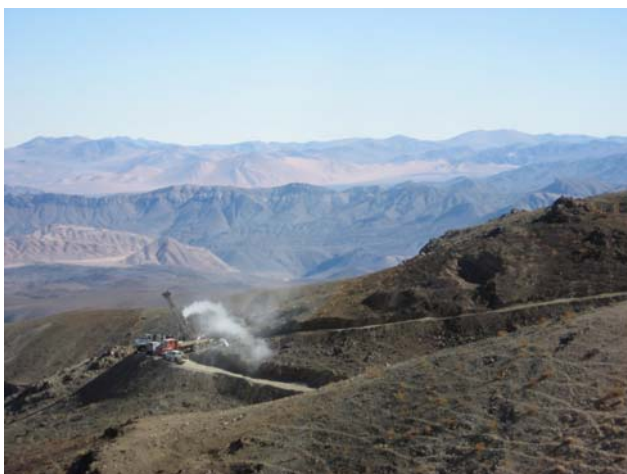
Figure 5: Reverse Circulation drilling at La Perla. The mineralised structure is to the right of the picture. The drillhole has been angled to intersect the structure at depth.
